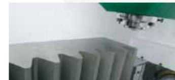
Collision protection system with the ability to detect impact forces of only 0.8 kg (8 N).
