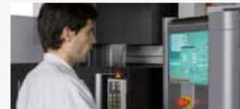
CNC-CAM capable of controlling up to 8 axes simultaneously, enabling CAD/CAM integration.
